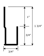
Both profiles provided in 6' lengths. One set of WCHANNEL will be two J-clips and one Z-Clip, enough to mount 6 linear feet of panels
